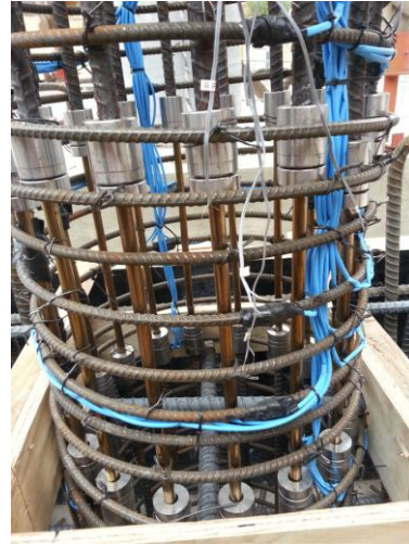
Figure 3. Reinforcing SMA bars used in plastic hinge
