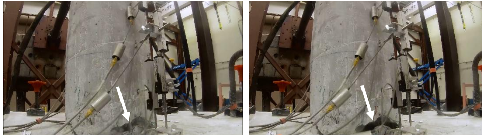
Figure 15. Tensile crack opening at the instant of maximum force during Runs 6 (left) and 7 (right).
