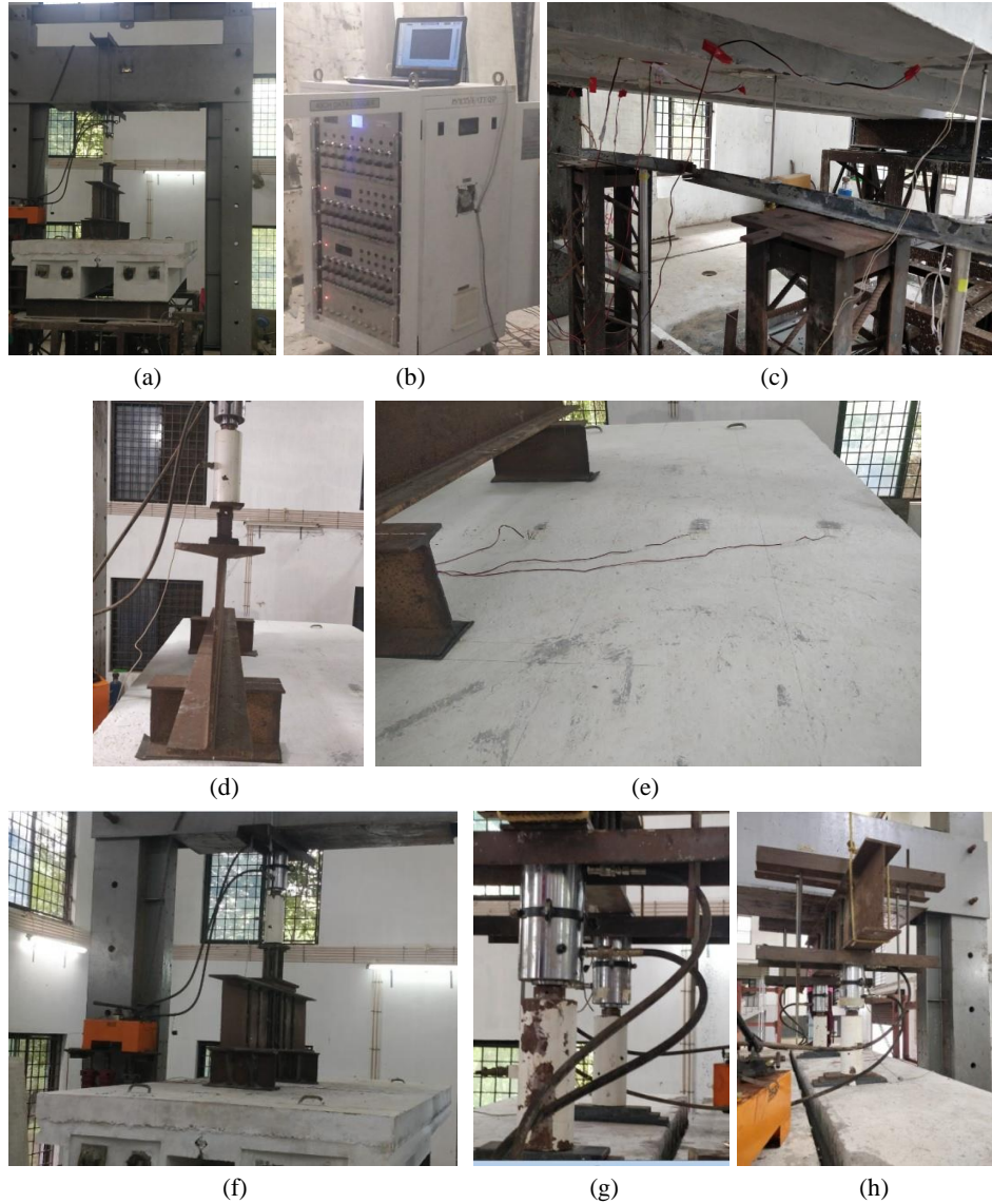
Photo 4. Arrangements in the order of load testing, a) Two point load testing arrangement, b) Data logger connected, c) Arrangement of LVDTs and Strain gauges at mid span, d) Close view of centralised load testing arrangement, e) Strain gauge fitted to compression, f) View of eccentric load testing arrangement, g) Enlarged view of load testing on PTGR1, and h) Load testing on PTGR2
