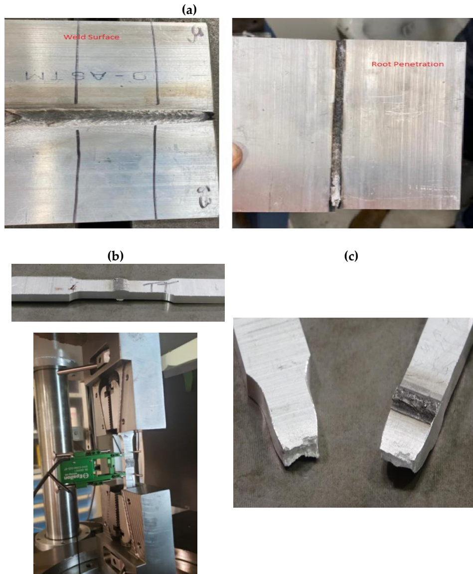
Figure 8. (a) Best sample of the 6.35 mm thickness for penetration (b) Schematic of the Force Measurement (c) Final sample after UTS measurement.
