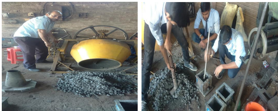
Figure 9. Cube making for test during experimentation
