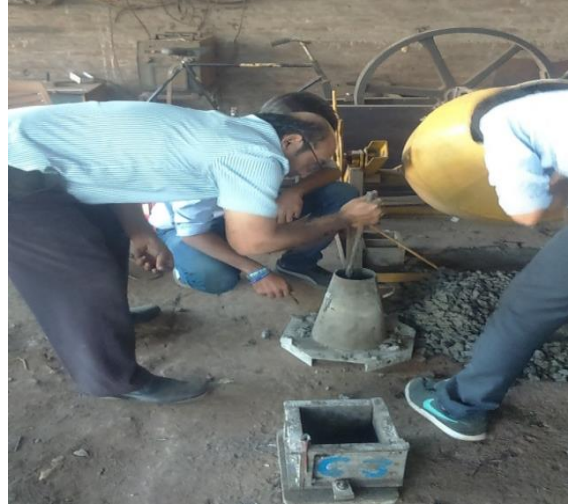
Figure 8. Execution of slump test during experimentation
