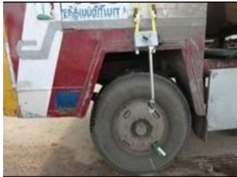
Figure 7. Auto clicker and reflector arrangement on the wheel
