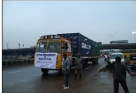
Figure 6. Truck employed for bridge testing
