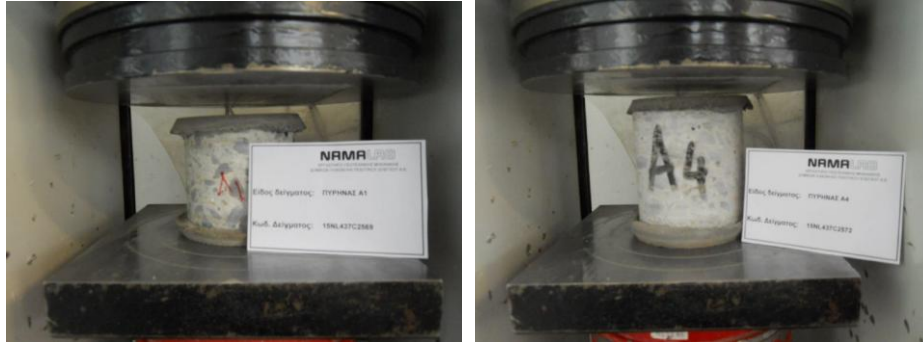
Figure 12. Cylindrical concrete specimens for evaluation of the material qualities
