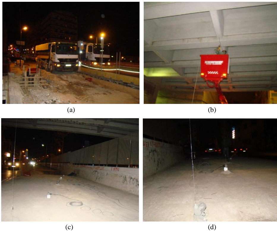
Figure 14. Test loading trucks and vertical deflection measurement devices
