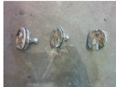
(b). Failed samples showing good bond
