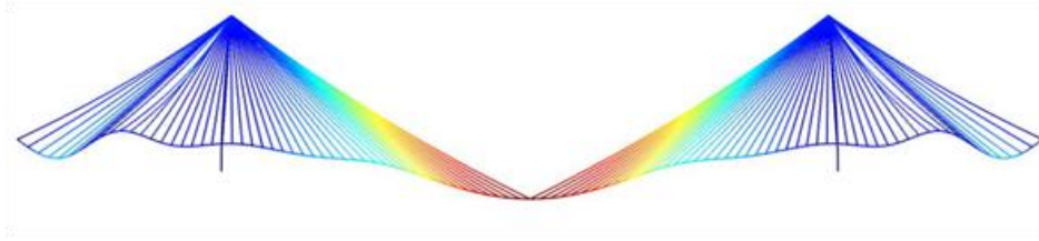
Fig. 9. Bridge deformed shape corresponding to the maximum load parameter for the NLM model in Fig. 8a.
