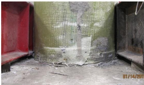
F4-24-P124-R: rupture of FRP wrapped layers
