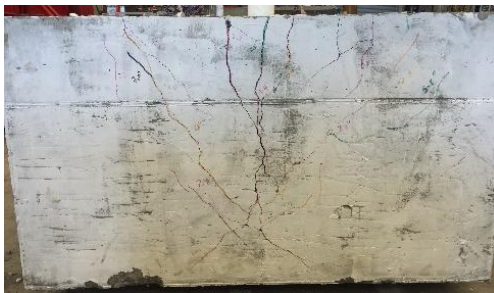
F4-24-E344: footing cone failure
