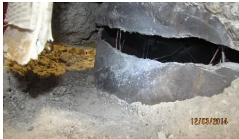
F4-24-E324-R: steel tube tearing
