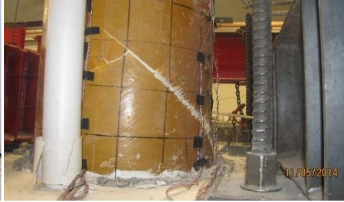
F4-24-E324: rupture of FRP tube
