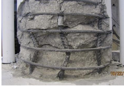
F4-24-RC: rebar fracture
