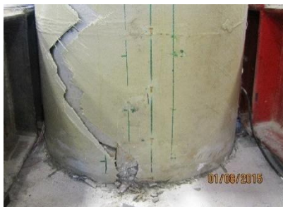
F4-24-P124: rupture of FRP tube
