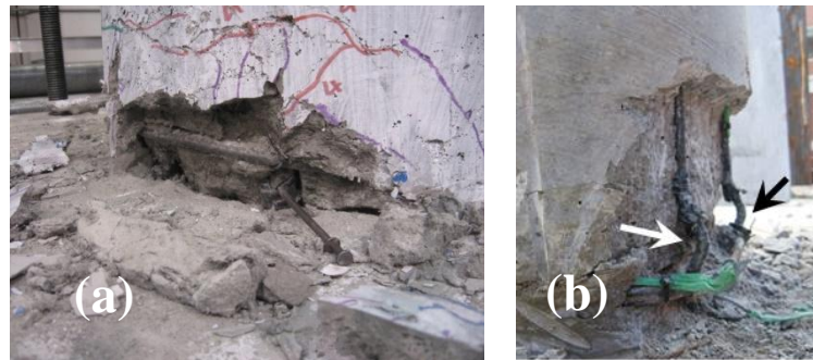
Figure 9. a) Rupture of longitudinal bars in RC-ECC, b) Buckled longitudinal bars in CFFT
