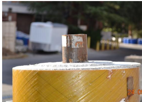
Figure 10. Condition of the pipe pin after test
