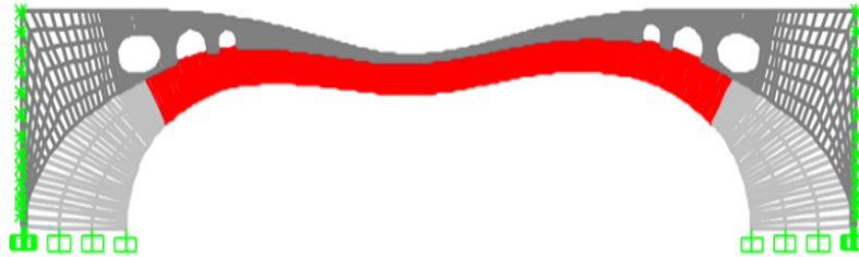
Figure 15. The deformed configuration of the bridge with fill with internal holes
