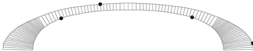
Figure 8. Asymmetric mechanisms with four unilateral hinges
